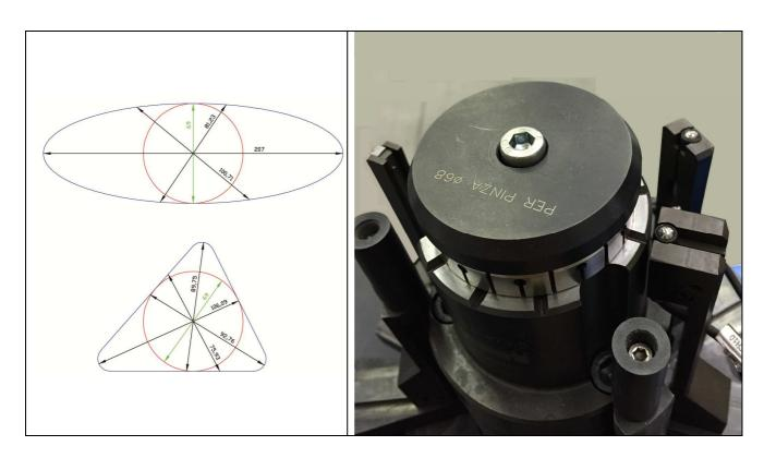
The solution patented by TQM ITACA TECHNOLOGY srl simulates the mounting condition; so the measurement made is correct and independent from the bore form.
