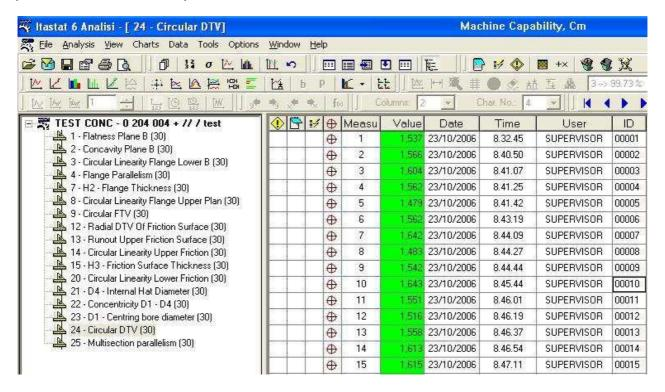
The following example is a report relative to disc S/N 00010, controlled on 23/10/2006 at 08:45:44. The disc was produced on the Kitako 2 production line and checked using the measuring station DF 2003 MMT S/N 00012-03.
