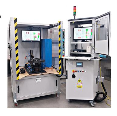
Itageo6<sup>©</sup> station for the control of brake discs in production line equipped by powered roller conveyor and linear system for the handling of pieces.
