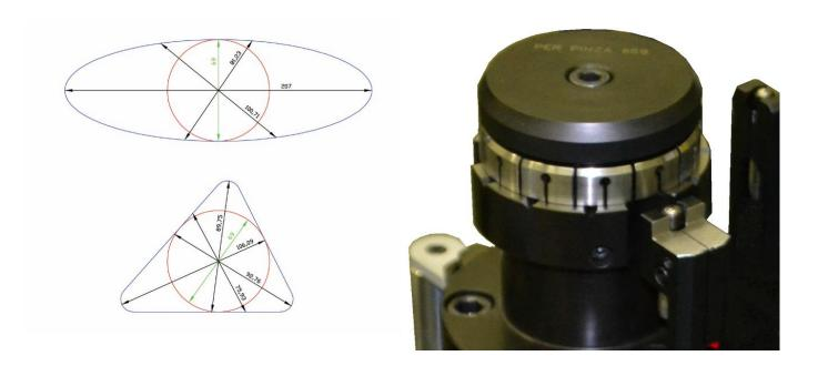
It's clear that with an error due to triangular form, the diameter measured by 2 counterposed probes is higher that the effective minimum diameter, with the risk of mounting problems.
