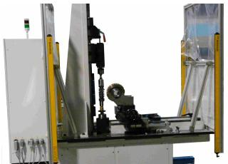
Itagear 6 station for the control of wheels and worm screws of big dimensions.
