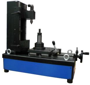
Gear inspection system for the control of gears on a shaft. Expansion plier for the locking of the master.
