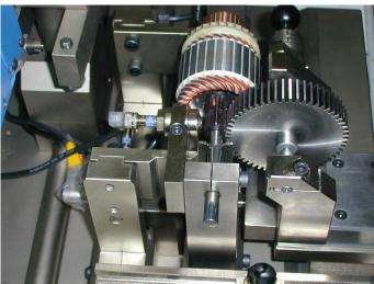
Itagear 6 station for the 100% control of machined gears on electric motors, with manual load/unload, movement forward of the sample wheel and automatic measuring cycle. The station is already fitted for the automatic load/unload.
