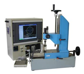
Itagear 6 complete station, with gear inspection system fitted for the control of gears on shafts and industrial PC with portable rack.
