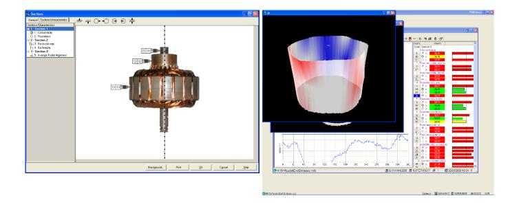
The result of the measuring is displayed as a polar profile and as a linearized graph with possibility of zoom. If necessary, it's possible to save the graphs of the single tests.
