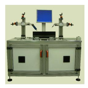
Semi-automatic bench for the control of brake pads for which it's necessary a precise impact point and a precise collocation of the microphone.
