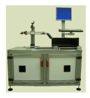
Semi-automatic bench for the control of pliers, brackets, supports, backplates, etc... with an innovative configuration system which guarantees an extreme repeatability of the test conditions: it's the ideal solution to test objects with a complex shape for which it's necessary to hit the part according to the specifications. Manual load/unload.
