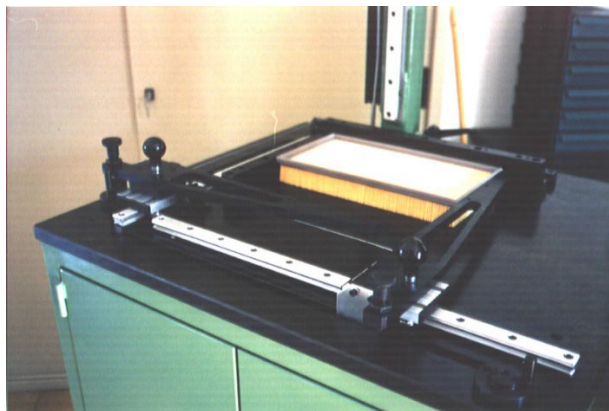
Itastat station for the dimensional control of the paper air filters.
